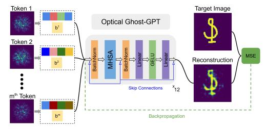
Figure 2: **Schematic of Optical Ghost-GPT**. The speckle patterns are first compressed into a latent space and then concatenated with the corresponding bucket measurements to form the input token sequence.
