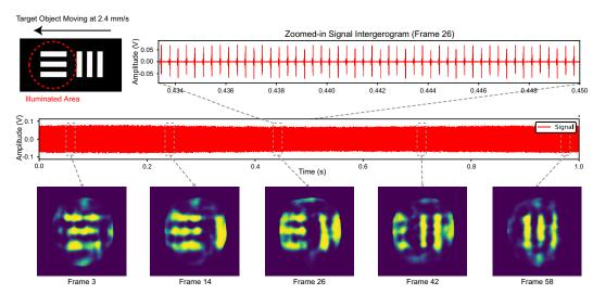
Figure 4: Video-rate image reconstruction of a moving target. A hyperspectral speckle pattern is projected onto a USAF1951 resolution target (Group 0, Element 4; 1.41 lp/mm), which is mounted on a motorized stage and translated horizontally at a speed of 2.4 mm/s.
