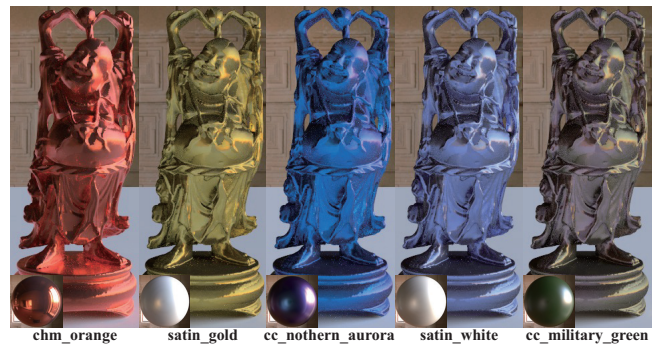
Figure 10: Editing specular colors \rho_s F of brushed_steel_satin_pink material by replacing those of isotropic materials (shown in the inset). Our method can change the specular colors without changing the shapes of highlights.
