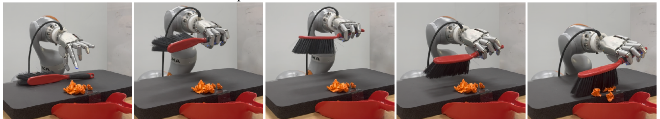
Fig. 1: SimToolReal is a framework for training a single general-purpose, object-centric RL policy in simulation and transferring it to real-world tool use. (Top) Zero-shot deployment on novel real tools and tasks, spanning thin markers to thick hammers. (Bottom) Tool use typically involves grasping objects from flat surfaces, reorienting them in-hand, and performing the task.
