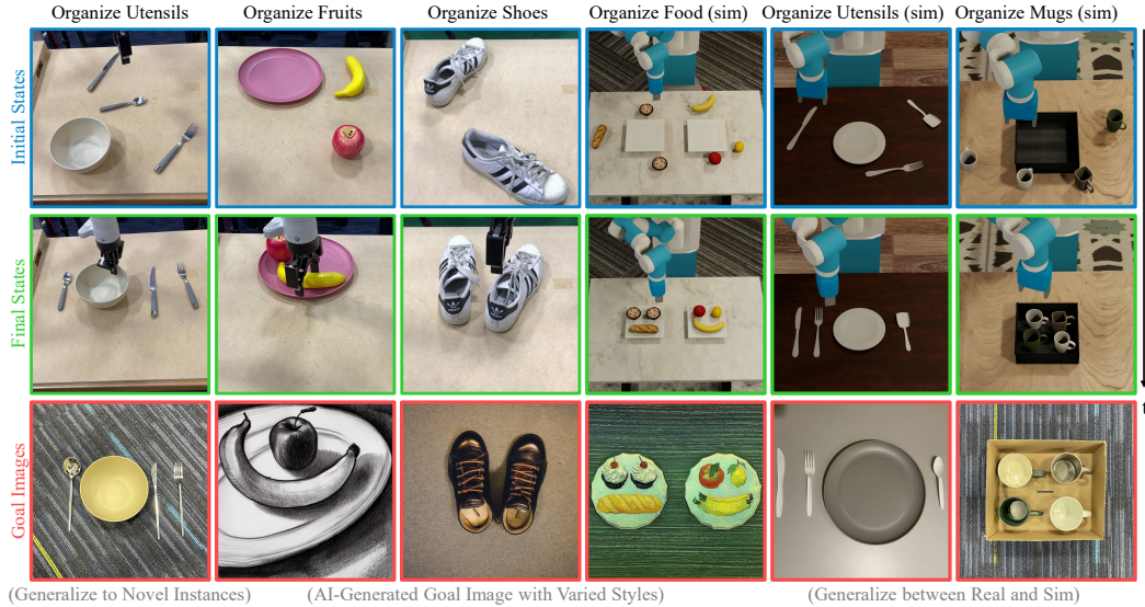
Figure 6: Qualitative Results. We qualitatively evaluate our proposed framework on rearrangement tasks, both in the real world and in simulation, encompassing tasks such as organizing utensils, fruits, shoes, food, and mugs. The figure highlights that our representation can generalize across varied instances, styles, and contexts. For instance, in the example of organizing fruit, the goal image, unlike the workspace, is styled as a sketch drawing. Because our representation encodes semantic features, the banana in the workspace can correspond with the banana in the goal image, which allows the task to be finished. This wide range of tasks showcases the generalization capabilities of our framework.
