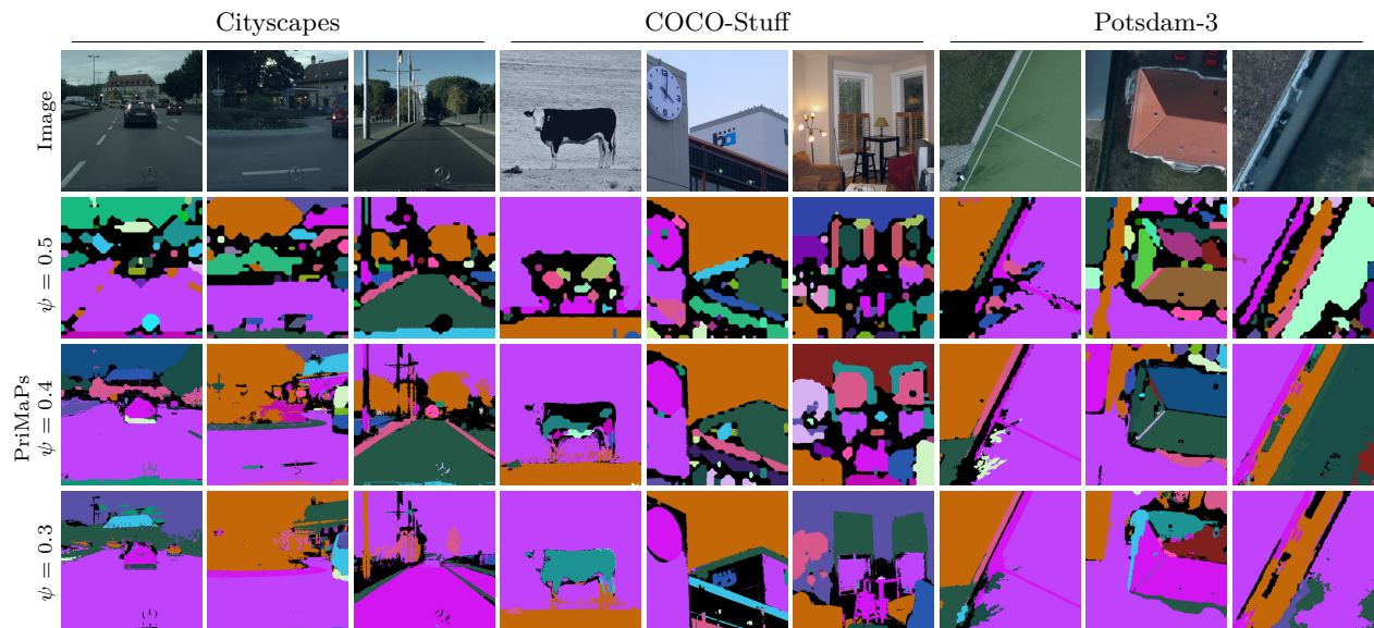
Figure 6: Qualitative threshold \psi ablation with DINO ViT-B/8 using different \psi values for PriMaPs mask proposal generation on all three datasets. The hyperparameter exhibits favorable stability properties.
