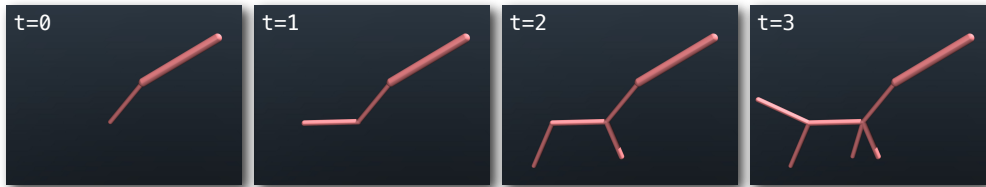
Figure 8: Designs process of Transform2Act for the 2D Locomotion environment. We visualize the design after each skeleton transform action. For better visualization, we use the joint attributes after the attribute transform stage.
