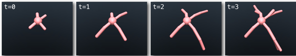
Figure 9: Designs process of Transform2Act for the 3D Locomotion environment. We visualize the design after each skeleton transform action. For better visualization, we use the joint attributes after the attribute transform stage.
