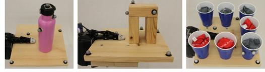
Fig. 4: Bottle, Arch, and Cups object arrangements used for experiments. The arch is an example of non-coplanar contact (the three blocks composing the arch are not attached together). The bottle is filled with sugar and the cups each contain bean bags instead of liquid to avoid spills in the lab.
