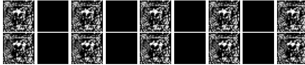
Figure 6: The odd columns plot the images generated by GAN with two randomly picked inputs \epsilon (the first and second rows, respectively) for different numbers of training iterations. From left to right, the images were sampled every 1K training iterations, starting from iteration 26K and continuing until iteration 30K. The even columns display the differences between the images on their two sides. The close-to-zero differences (as suggested by the black patches) indicate that the GAN’s outputs are nearly unchanged.
