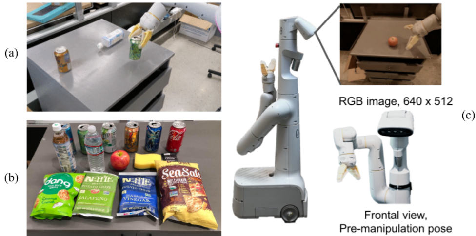
Figure 3: (a) A mobile manipulator robot performs a variety of manipulation tasks with various objects and cabinet drawers in an office kitchen environment. (b) An example of some of the kitchen objects found in the demonstration dataset. (c) The mobile manipulator robot receives RGB images from an over-the-shoulder camera and uses a 7 DoF arm with parallel-jaw grippers.
