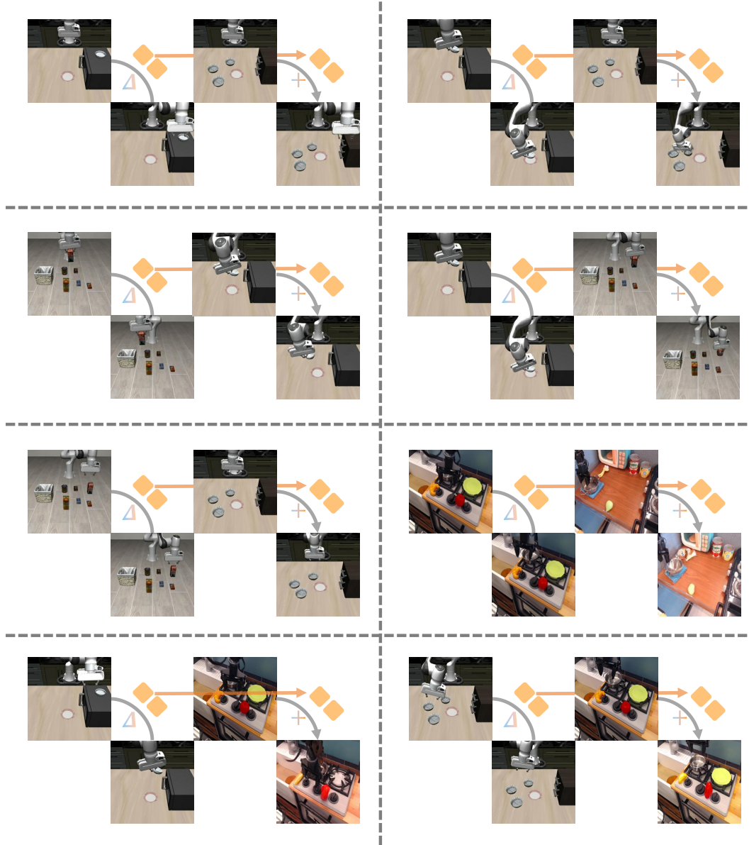
Figure 8: Transfer linear interpolation experiment with the StaMo encoder. The left and right panels illustrate different task scenarios, where reconstructions are obtained by \text{tokens}(3) + \text{tokens}(2) - \text{tokens}(1) , demonstrating the linear interpolation property of latent representations during transfer.
