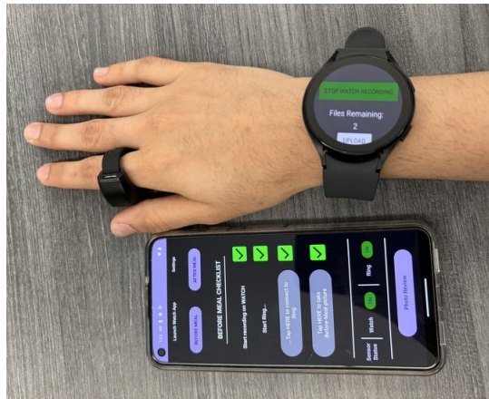
Fig. 2. Smart ring, smartwatch, and smartphone used for recording data with MealWatcher toolset.
