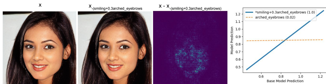
Figure 8: Comparison with the Wachter counterfactual generation method. A smiling classifier with a known bias of arched_eyebrows is used to observe if this bias can be detected. The Wachter counterfactual doesn’t appear to modulate the input image in a human interpretable way, instead many small swirls appear on the face which change the prediction for smiling but not for arched_eyebrows .
