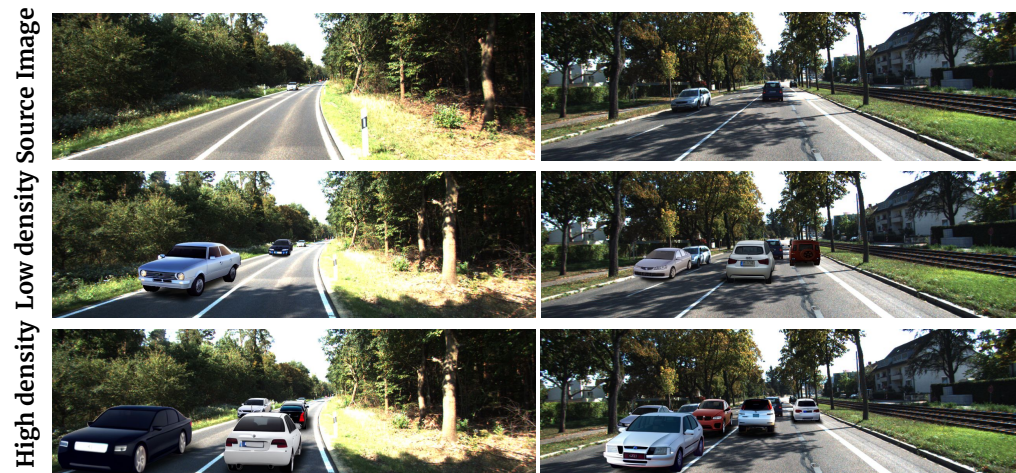
Figure 8: Augmented training dataset for 3D object detection: Given a sparse scene with few cars, we place cars at the predicted 3D bounding box locations using our rendering algorithm. We present two sets of results, one with low density (1 – 3 cars added) and another with high density (4 – 5 cars added) for each scene.
