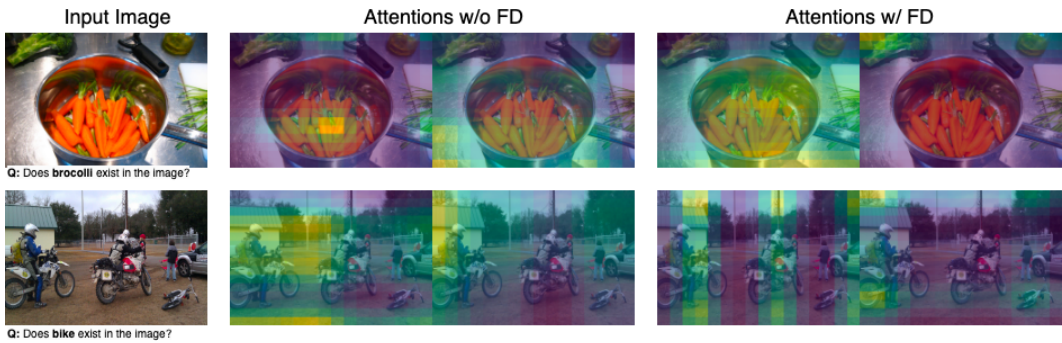
Figure 3: Visualization of feature maps with and without FD. We select one query in the perceiver resampler and visualize its attention map in two fixed heads over the image. With FD, the attention maps not only show higher diversity but also focus more on informative and fine-grained regions (e.g., broccoli in the first row and bike in the second row).
