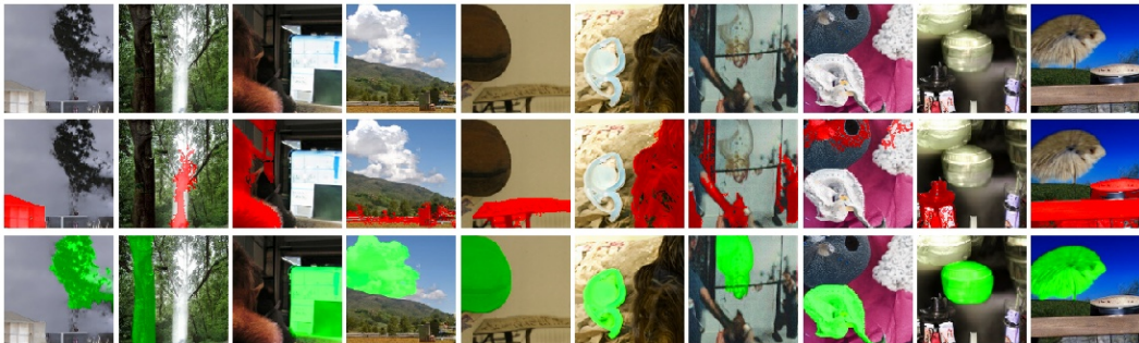
Figure 8: Failure cases of masks generation. Top : BigBiGAN samples; Middle : masks produced by latent manipulations; Bottom : masks produced by the supervised saliency model.
