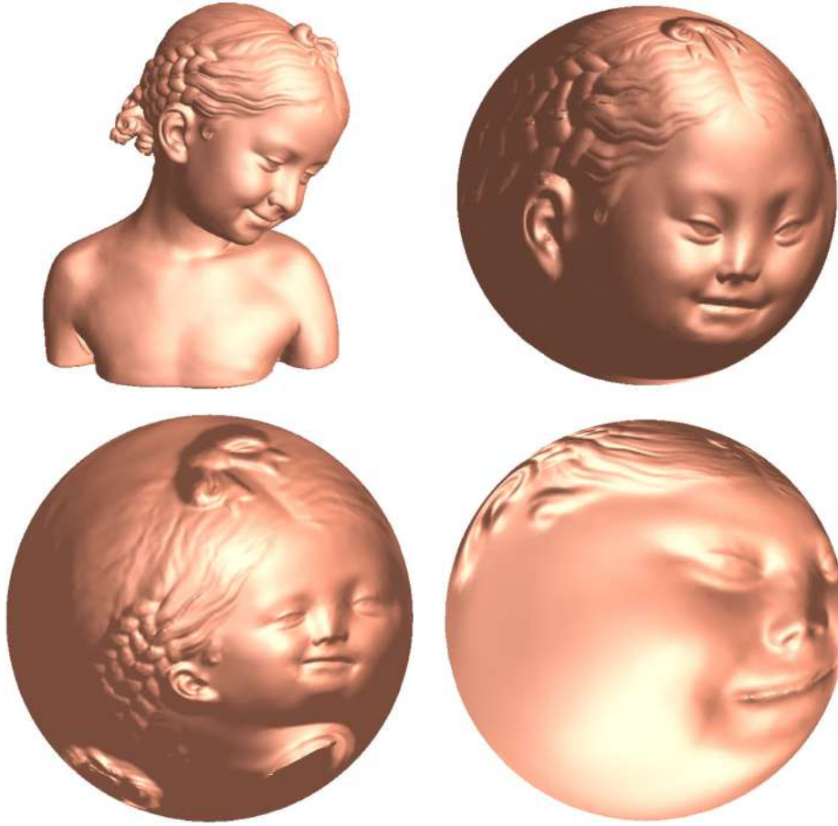
Fig. 1. The bimba surface is conformally mapped onto the unit sphere. The mapping is unique up to a Möbius transformation.
