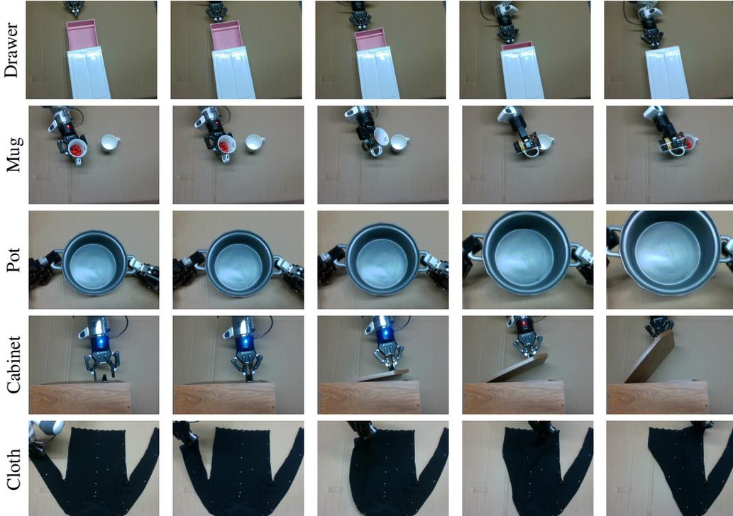
Figure 6: **Real robot experiments** We show the visual observations of the real robot for the five unseen objects from drawer closing task to cloth folding task.
