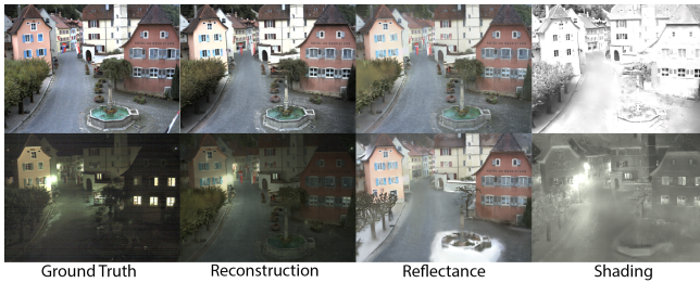
Fig. 8. Time Splatting for Traditional Time-Lapse: To demonstrate the applicability of time splatting to traditional time-lapses, we perform intrinsic image decompositions on the SkyFinder [Mihail et al. 2016] dataset. Time splatting separates seasonal information like snow in the reflectance image and lighting effects in the shading image.
