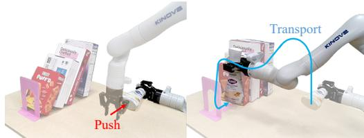
Figure 1: The robot places an object into a cluttered shelf by exploiting object interactions. It uses the grasped object to manipulate other objects within the shelf through pushing and sliding actions and finally places all the objects in the appropriate location.
