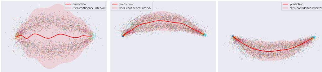
Figure 11: Results of GMR on multimodal demonstrations and single-mode demonstrations. Left: Prediction with 95% confidence interval from a GMR trained on multimodal demonstrations. Middle/Left: GMR predictions on single-mode demonstrations.
