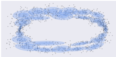
Figure 14: GMM model for the multimodal demonstrations recorded using motion tracker.
