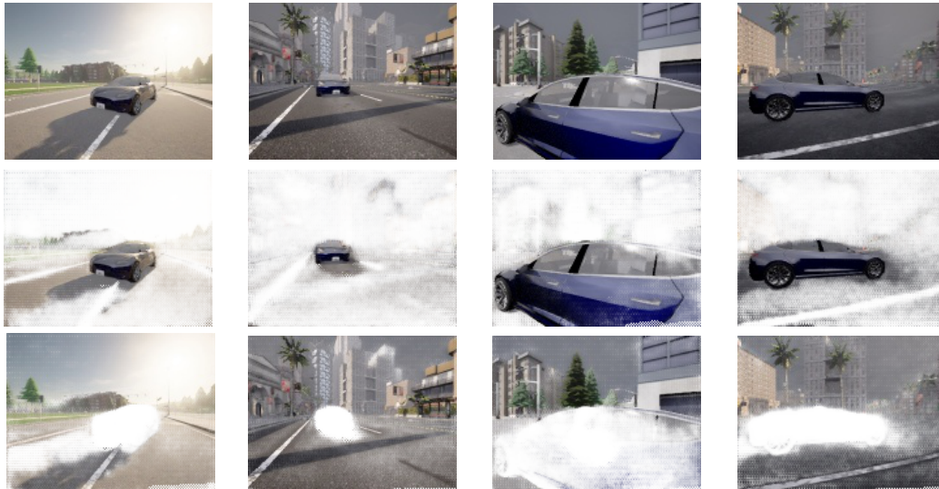
Figure 5: Segmentation performance on images of cars in virtual towns generated by Carla. Top: input images, middle: image weighted by the inferred mask for the object slot containing the car, bottom: image weighted by the inferred mask for the background. Other slots (3 in total in training) are neglected.
