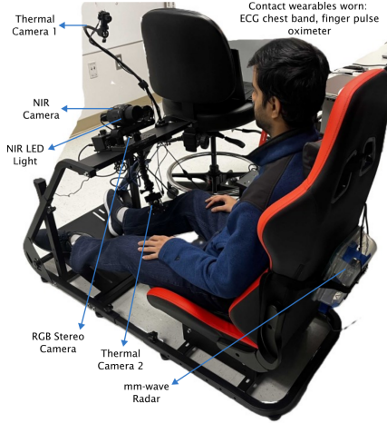
Figure 2: CogPhys Multi-modal capture setup. We record signals from seated participants using various non-contact sensors (RGB Stereo camera, NIR camera, two thermal cameras, mm-wave radar) and contact wearables (chest band for ECG and respiratory signals, and finger pulse oximeter). The participants perform several tasks, such as sitting still, reading, performing arithmetic operations, etc., while the signals are recorded.
