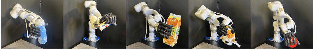
Figure 7: Zero-shot deployment of our method on an xArm with an Ability Hand. Our model directly transfers to the real world from simulation, successfully executing open-loop grasps across a variety of everyday objects using point cloud input.
