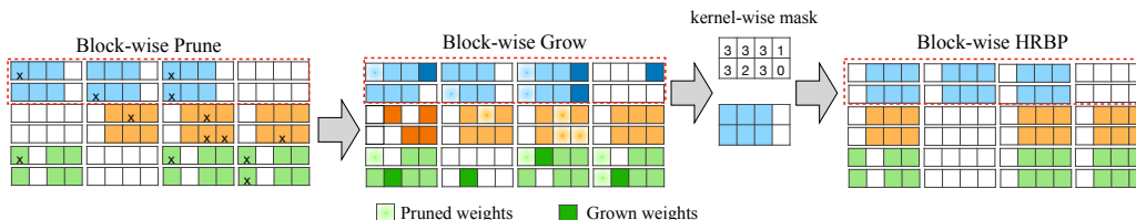
Figure 4: Block-wise updating for Dynamic Sparse Training. Take the block with blue color as an example, for each row, we prune 2 weights (crossed cells) based on magnitude and grow back 2 inactivated weights (darker cells) based on gradients. We then rerun HRBP to identify a new dense block for each group by generating kernel-wise masks to determine the kept kernels and applying pattern findings within each group.
