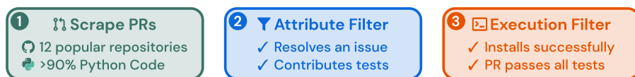
Figure 2: SWE-bench task instances are created from merged pull requests that resolve an issue, contributes tests, and install successfully.
