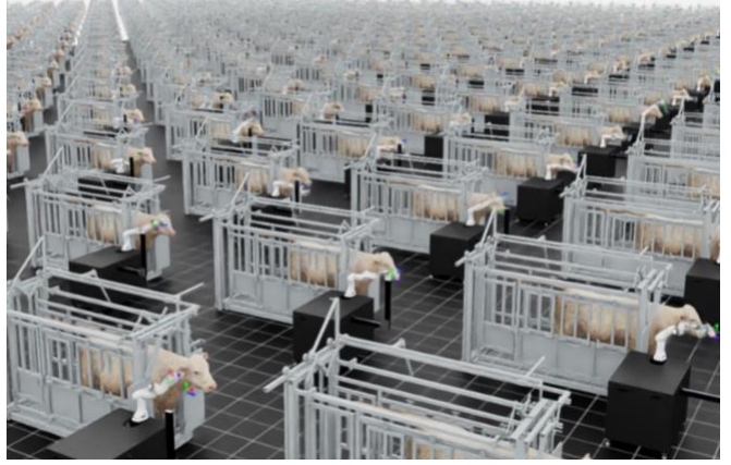
Fig 1 The training environment in NVIDIA Isaac Sim, showing the digital twin of the robotic arm, cattle, and chute used to train the reinforcement learning agent
