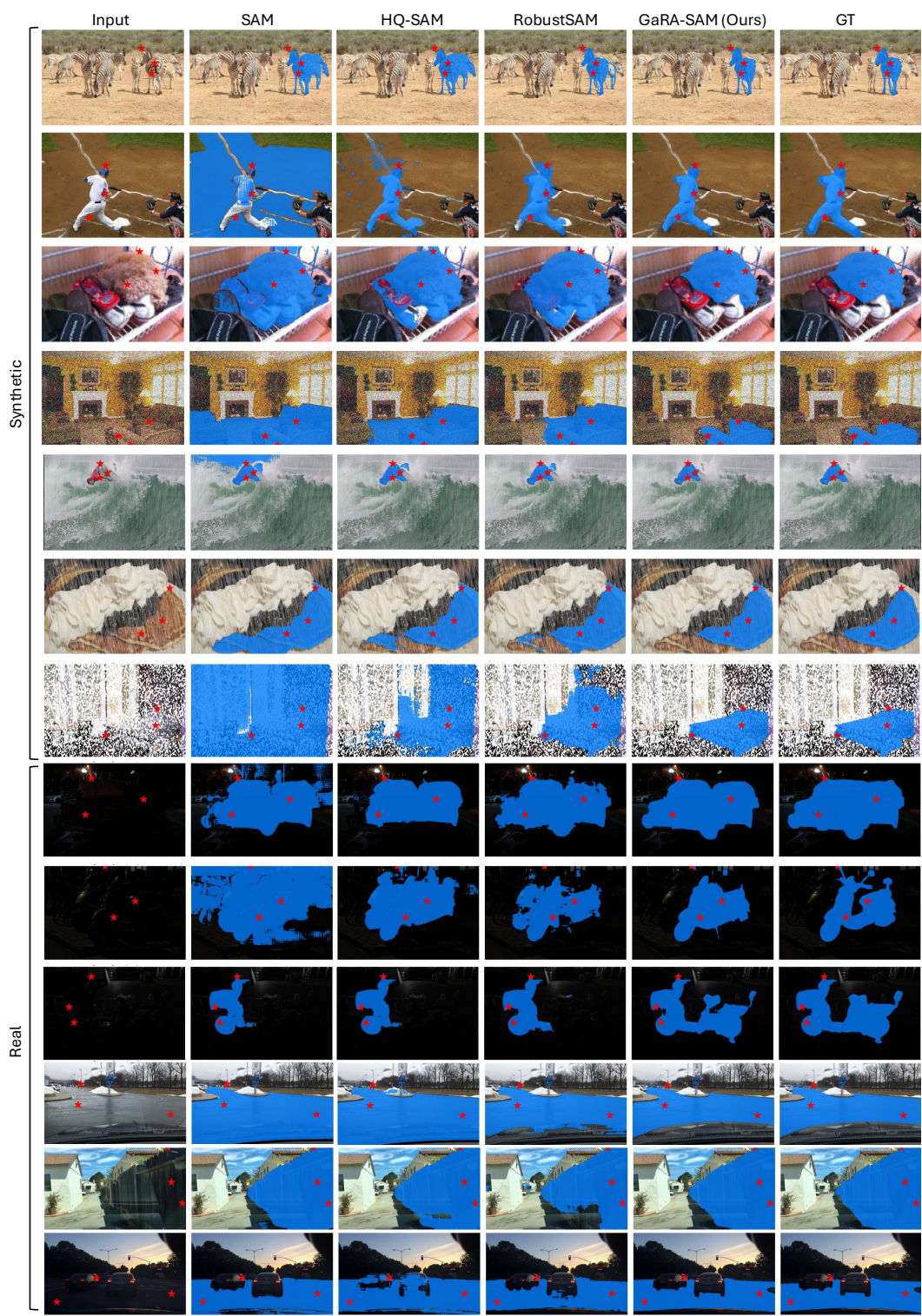
Figure a3: Qualitative results under both synthetic (top) and real-world (bottom) corruptions. From left to right: input image, SAM, HQ-SAM, RobustSAM, our method GaRA-SAM, and the ground truth (GT). GaRA-SAM consistently produces more accurate and complete segmentations, particularly under challenging conditions such as noise, blur, and low-light scenarios.
