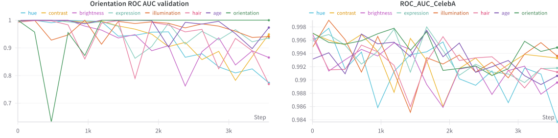
Figure 16. Left ROC AUC curve for ArcFace resnet 18 measured on a monovariant dataset of orientation variations. We see that the model fine-tuned on orientation performs the better. Right Along finetuning performance on CelebA decreases, but stays at a decent level.
