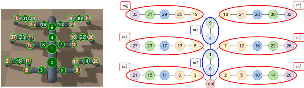
Figure 1: Graph Structure and Neural Network Modules of the 6 Leg Centipede. Left: The robot’s joints are labeled numerically and circled. Right: The joints form the nodes and the links are the edges. The subset of joints that form each leg module are circled in red, while those that comprise each body module are circled in blue. Neural network modules are denoted as m_k^i , where k refers to the type, e.g. all leg modules are type 0, and i denotes different instances of the same module type.
