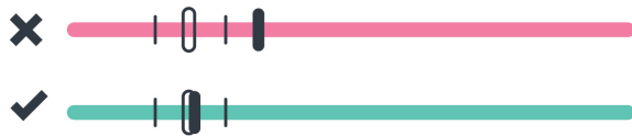
Figure 3: Slide control for transmission and feedback of the user input. The dark line element indicates the direction. If it is within the tolerance range (thin lines / contour), the display is green (bottom). Outside this range, the display turns red (top).
