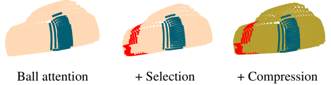
Figure 2. Receptive field visualization of a car in the ShapeNet dataset with different components: ball attention; ball attention and selection; ball attention, selection and compression. The receptive field increases with more components.
