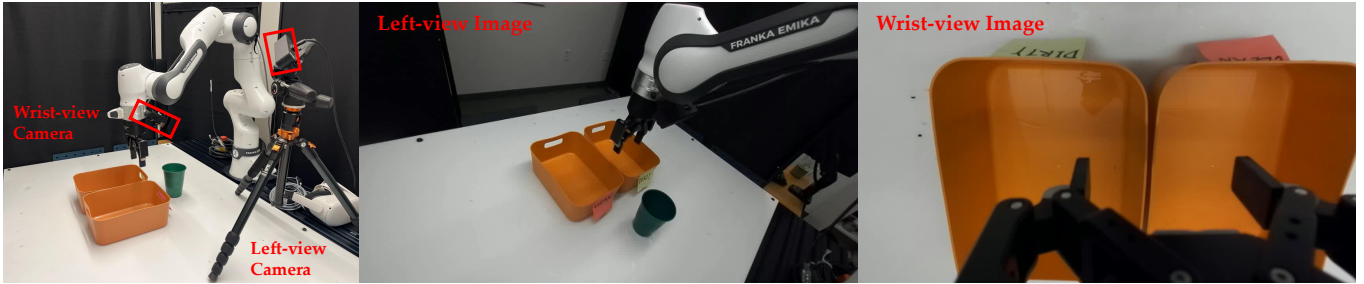
Fig. 8: Hardware Setup. We demonstrate our hardware environment setup with a Franka Emika Panda arm and two Zed cameras (left image). In the middle, we show the left-view image captured by a Zed 2i camera and on the right, we show the wrist-view image captured by a Zed M camera.
