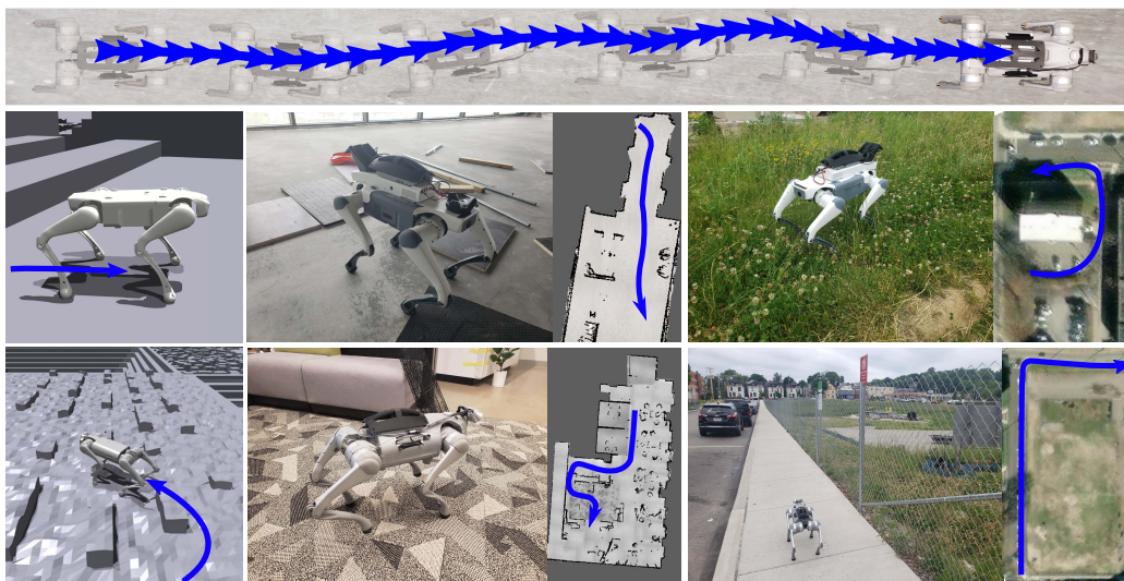
Figure 1: Robot state estimation by Legolas across diverse environments and robotics platforms. Legolas operates at a high frequency to predict small incremental motions of a robot by only utilizing leg and IMU sensing. We introduce the first accurate, purely data-driven method for predicting odometry.
