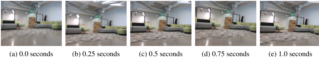
Figure 6: Quick motions and large changes in rotation occurring over one second. These quick motions cause degraded image captures on the quadruped affecting the deployment of the visual baseline. Changes in pitch (Fig. 6a,6b,6c,6d,6e) and roll (Fig. 6a and Fig. 6e) are notable.
