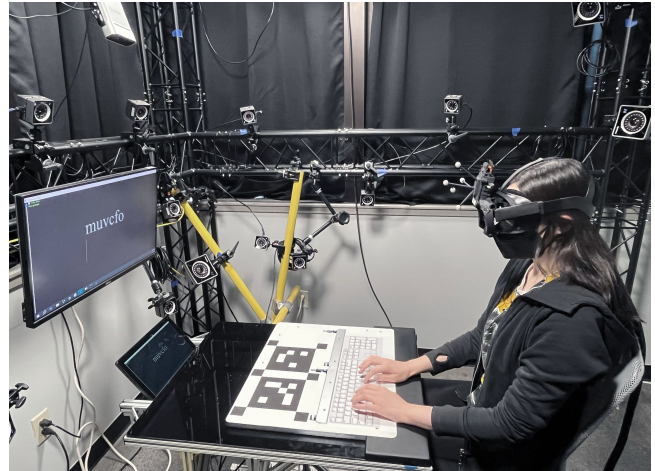
Figure 2: A data collection setup with a typist sporting a head-mounted stereo camera rig. The user is typing on a touchpad keyboard in front of a monitor that displays the transcription prompts and their typed text.
