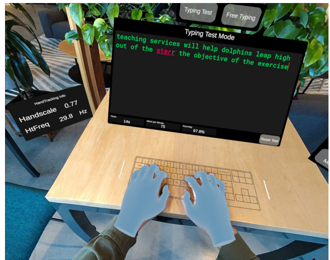
Figure 1: A person in mixed reality performs a transcription task on a virtual keyboard superimposed on a flat surface, with StegoType mapping hand motion into typed keys.
