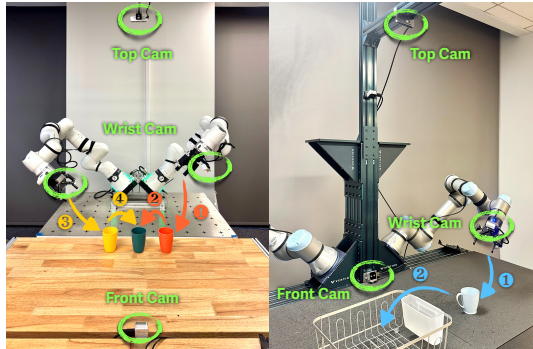
Figure 8: Real-world experiments setup. Left: Cup Stacking on Franka. Right: Cup Placing on UR5.
