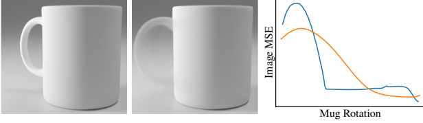
Figure 2. Optimizing the cup’s rotation in the hard (left, blue) and smooth (right, orange) setting (note the blurred handle). The image-space loss is displayed on the right: blurring removes the plateau.
