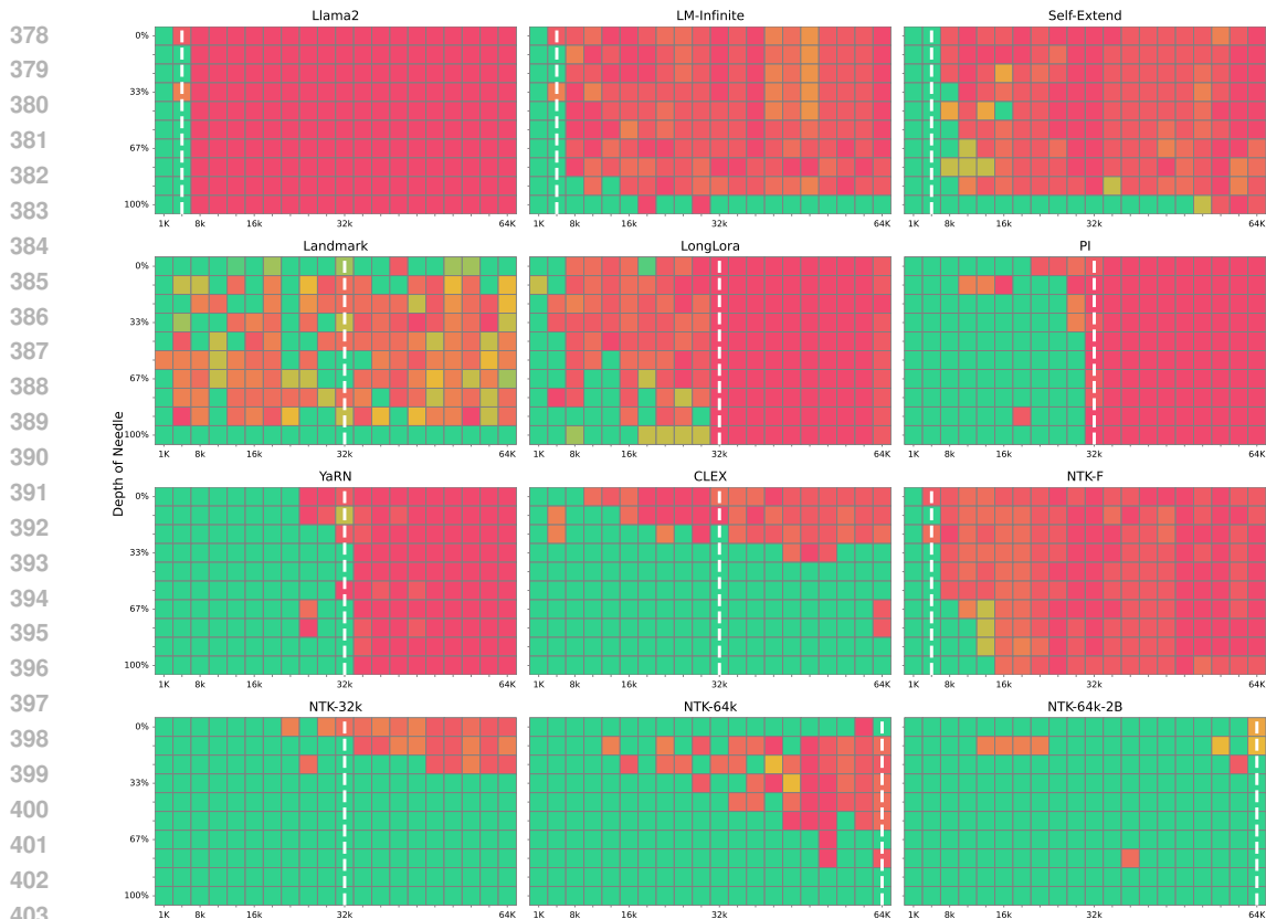
Figure 1: Needle in a Haystack evaluation. Green squares indicates a high retrieval success rate, the white dashed line denotes the longest length examples seen at training or finetuning, and the Y-axis represents the distance to the retrieved target.
