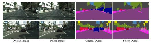
Figure 4: Visualization of images and models' predictions on them. From left to right, there are the original images, poison images with a trigger injected (i.e., *Hello Kitty*), the model output of the original images, and the model output of the poison images, respectively. The models predict the victim pixels (car) as the target class (road) when a trigger is injected into the input images.
