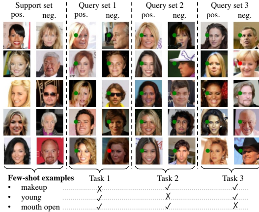
Figure 2: Visualization of classification of three different classifiers sampled from a trained VMAML-info. Left two columns show the support set \mathcal{D}_u^S , while other columns show images for each of the three ambiguous modes of the tasks. Each image is marked with either green dot if the predicted classification was correct or red otherwise.
