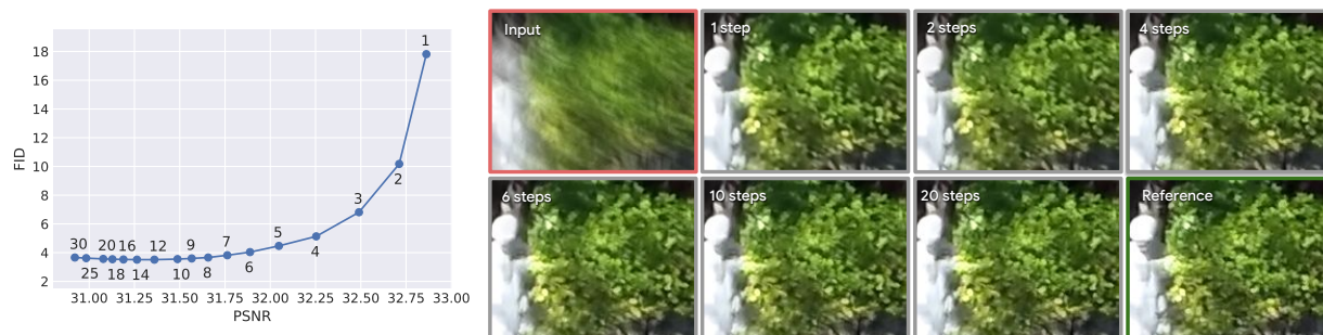
Figure 3: Number of steps. The total number of steps in the iterative regression has a direct impact on the quality. The number of steps seems to control the Perception-distortion tradeoff. One step leads to the best possible MSE reconstruction (minimum distortion) but large perceptual discrepancy.
