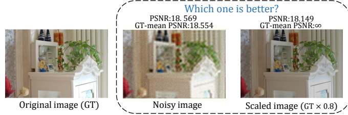
Figure 2: A comparison between the noisy image (obtained via by removing some Fourier high-frequency components and adding Gaussian noise) and the scaled image (the original image’s brightness scaled by a factor of 0.8). Taking a zoomed-in view, it is obvious that the scaled image exhibits significantly better quality. However, the PSNR values of the two images are comparable, posing challenges to this most commonly used metric for evaluating LLIE’s performance. In the contrary, their GT-mean PSNR values present huge difference, aligning with the true condition. For the scaled image, GT-mean PSNR is computed as PSNR(\frac{\mathbb{E}[GT]}{\mathbb{E}[GT \times 0.8]}, GT \times 0.8, GT) , resulting in an infinite PSNR value (In practice, PSNR usually has a pre-defined upper bound. In this figure, we strictly follow the mathematical definition of PSNR for demonstration purposes).
