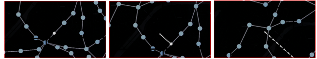
Figure 4. Close-up of SlidingRing (combined view). From left to right: as the user moves its field of view away from the link the ring is attached to, the trail (dashed line) guides the viewer back to the link, even when the ring is no longer in the AR view (right).
