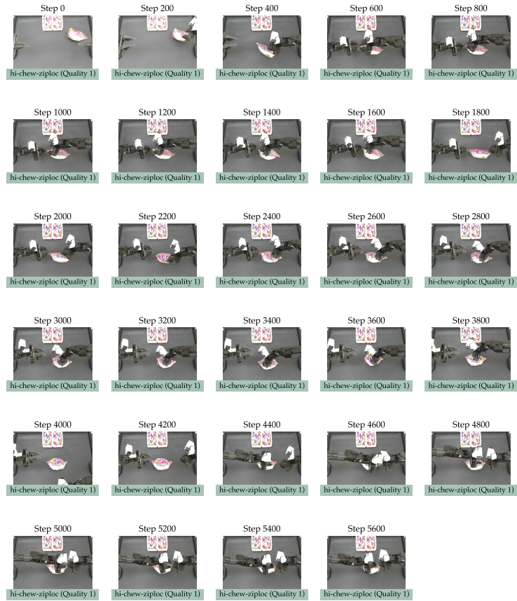
Figure 7: In this trajectory, the user correctly moves the Ziploc from the corner of the table to the center of the table, and grasps a Hi-Chew from inside the Ziploc which they bring to the End Zone. They are unsuccessful in closing the Ziploc before episode termination. The user is task-directed for the whole episode, however takes longer than better quality trajectories for this task and performs retrying behavior at each subtask. The whole trajectory is marked as hi-chew-ziploc (Quality 1).
