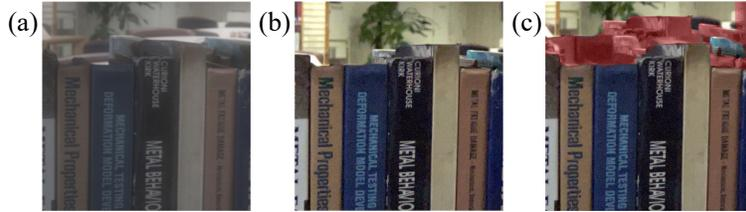
Figure 7: Invalid mask visualization in Feng-R [13]. (a) The degraded image captured by the ZTE Axon 20 [10] UDC. (b) The ground-truth image captured by the iPhone 13 Pro rear camera [25]. (c) Aligned ground-truth image by AlignFormer [13].
