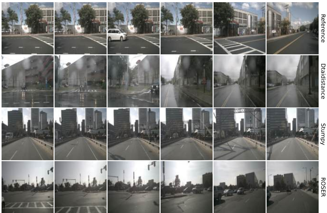
Figure 35: nuScenes qualitative results for right turn maneuver. ROSER and Dtaidistance successfully retrieves similar task while Stumpy retrieves a straight driving scene.
