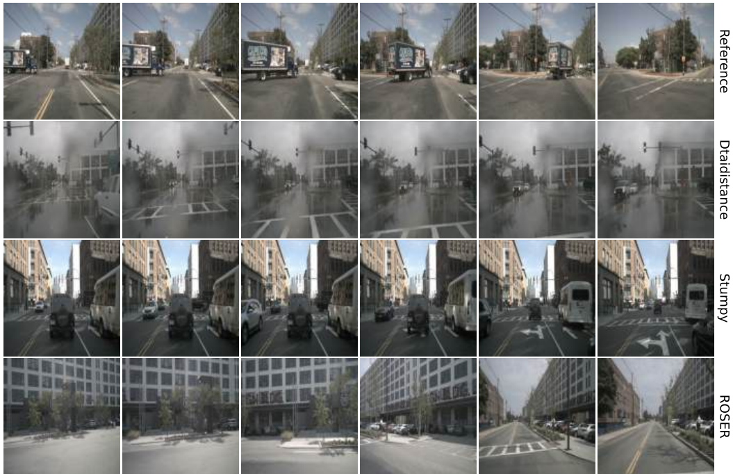
Figure 33: nuScenes qualitative results for left turn maneuver. ROSER successfully retrieves similar task while Dtaidistance retrieves a regular stop and Stumpy retrieves a straight driving scene.
