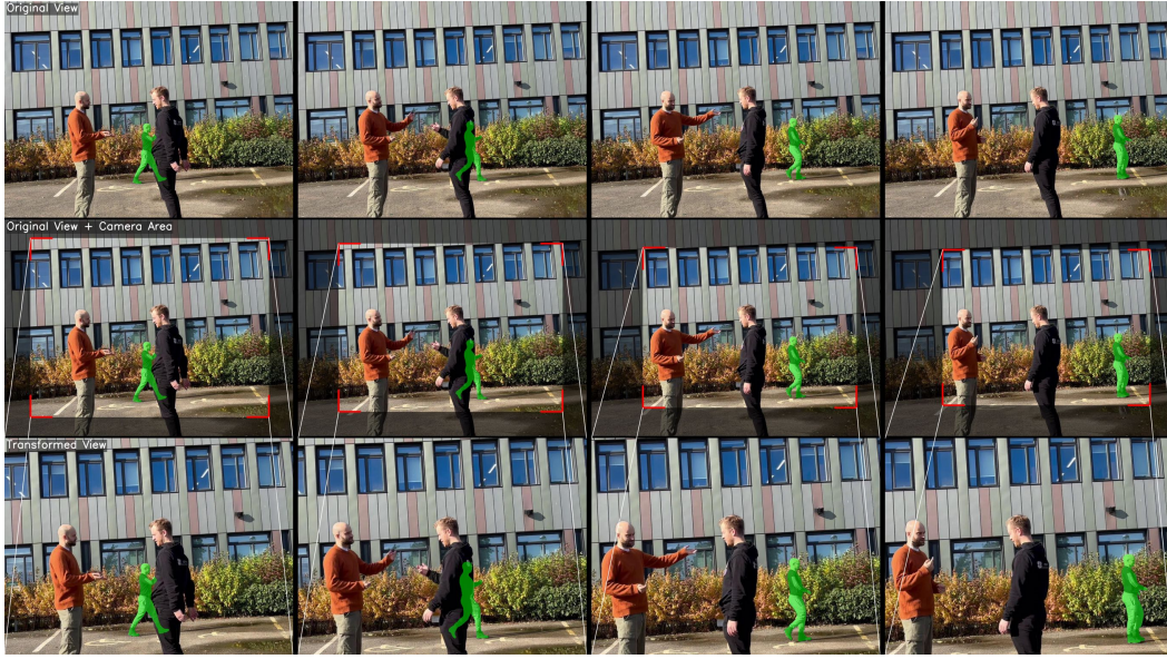
Figure 4: An example of an emulated camera motion. This figure demonstrates a dynamic zoom and pan by showing the original frame, the specific sub-region that constitutes the new camera view, and the resulting transformed frame.
