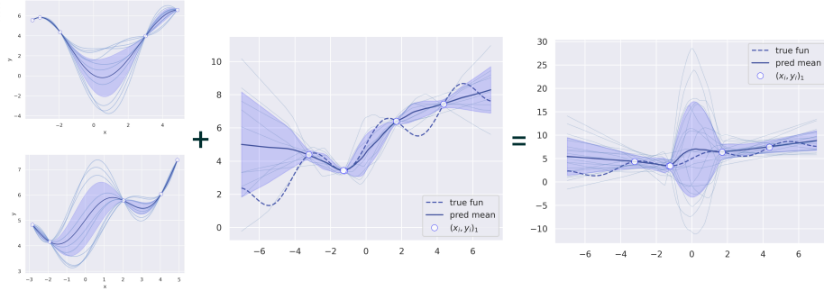
Figure 6: MARS prediction on samples from the sinusoid environment, with no data in the [-2, 2] range. Left: posterior predictions of two randomly selected GPs fitted to the meta-tasks. Middle: fBNN predictions, fitted using s_\phi^\mu , the score estimation network trained on GP mean predictions. Right: fBNN predictions, fitted using s_\phi , the score estimation network trained on samples from the GPs. Training fBNN with s_\phi (by sampling from the GPs) successfully incorporates uncertainty about the [-2, 2] part of the input domain.
