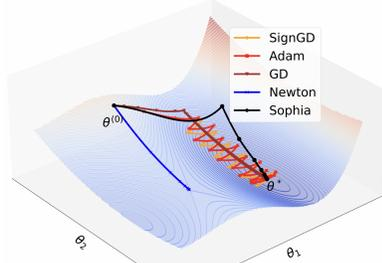
Figure 5. The motivating toy example.  $\theta_{[1]}$  is the sharp dimension and  $\theta_{[2]}$  is the flat dimension. GD’s learning rate is limited by the sharpness in  $\theta_{[1]}$ , and makes slow progress along  $\theta_{[2]}$ . Adam and SignGD bounce along  $\theta_{[1]}$  while making slow progress along  $\theta_{[2]}$ . Vanilla Newton’s method converges to a saddle point. Sophia makes fast progress in both dimensions and converges to the minimum with a few steps.
