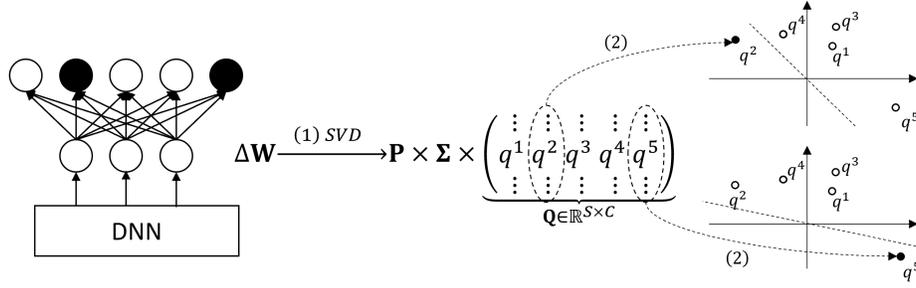
Figure 1: An illustration of RLG. Black nodes correspond to labels of samples used to compute the weight update. (1) The weight update of the projection layer  $\Delta\mathbf{W}$  is decomposed into  $\mathbf{P}\Sigma\mathbf{Q}$  by SGD. (2) Each column in  $\mathbf{Q}$  is mapped to a point in an  $S$ -dimensional space. If a point is separable from the rest, the corresponding label is predicted as being included in  $\mathcal{S}$ .
