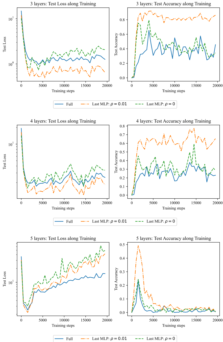
Figure 20: Synthetic IOI trained with Adam : test loss and accuracy for transformers with layers L = 3, 4, 5 . Truncating the last-layer MLP’s input weights with \rho = 0.01 improves the test performances for L = 3, 4 , while the model fails to converge for L = 5 .
